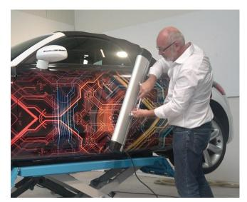
heat them again after the wrapping process, without rubbing them again. This can be done with a heat gun or with a heat lamp. The car body should be heated up to a temperature of 70 to 90 °C).
